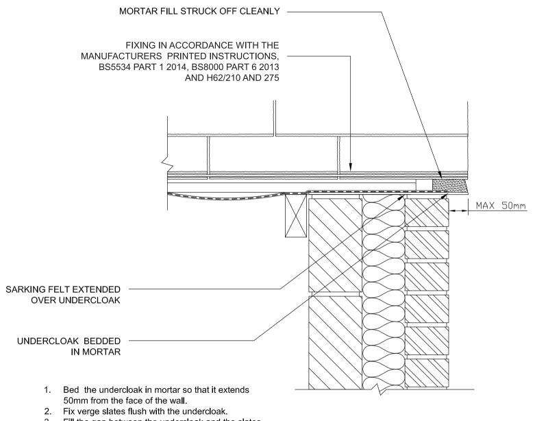
3. Fill the gap between the undercloak and the slates with mortar and strike off smoothly to provide a flush joint and cut back joint as shown.
